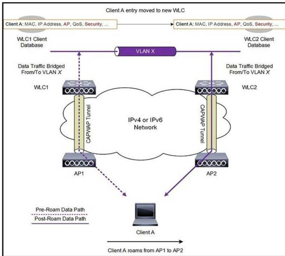
A client roams between two APs that are registered to two different controllers, where each controller has an interface in the client subnet. Both controllers are running AireOS.
