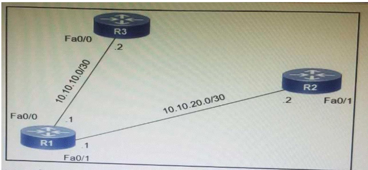
An IP SLA was configured on router R1 that allows the default route to be modified in the event that Fa0/0 loses reachability with the router R3 Fa0/0 interface.
